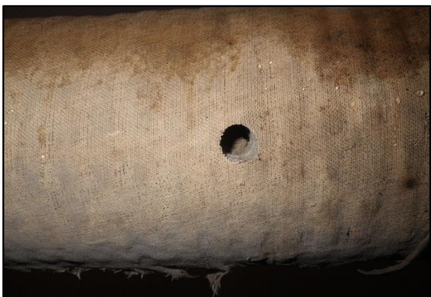
11. The aluminum cutter sleeve allows full depth sampling even for denser materials such as the wrapped layers of paper that make up woolfelt pipe insulation. This ensures accurate sampling even when asbestos may only be present on the inner layer of the pipe insulation.
