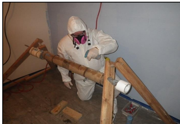
8. The individual conducting the asbestos core sampling using the Wonder Makers Asbestos Bulk Sampler had two asbestos air sampling cassettes positioned in his breathing zone area during the sample collection process. Personal sampling pumps were worn on the sample collector's belt attached with tygon tubing to the asbestos air monitoring cassettes. The sampling was done according to EPA guidelines and manufactures instructions, including the pre-sampling step of wetting the material to be sampled.
