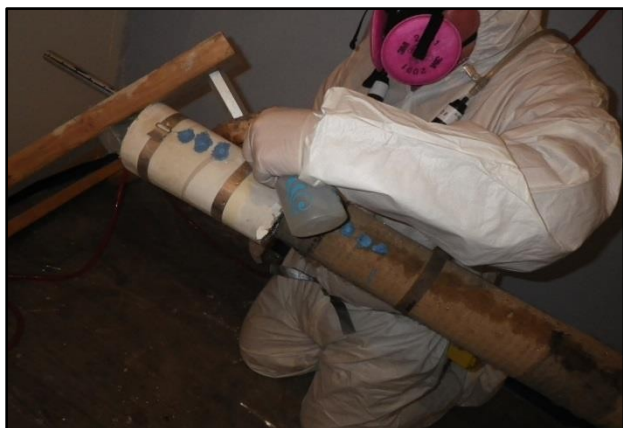
9. A small spray bottle of surfactant was used to wet the asbestos-containing pipe insulation at the point where the asbestos bulk sample was collected with the Wonder Makers Asbestos Bulk Sampler.
