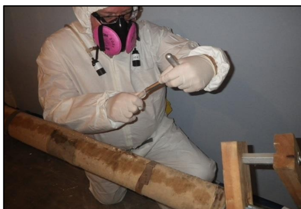
12. After each core of asbestos was extracted from the pipe insulation, the cutter sleeve and sample were both placed into the plastic collection vial that comes with every cutter sleeve.
