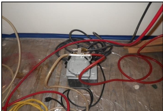
7. A Triple-Air High Volume Air Sampling Pump manufactured by Wonder Makers was also used to collect representative air samples during the collection of bulk samples. As its name implies, this pump was able to collect air samples in three locations within the simulated boiler room while the aircell and woolfelt insulation was being sampled.
