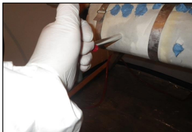
10. The Wonder Makers Asbestos Bulk Sampler Aluminum Cutter Sleeve was used to core into the asbestos-containing pipe insulation to collect a full depth sample of the pipe insulation.
