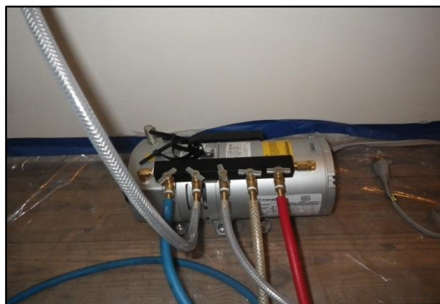
6. A Multi-Air High Volume Air Sampling Pump manufactured by Wonder Makers was used to collect representative air samples in five locations within the simulated boiler room during the asbestos sampling process.
