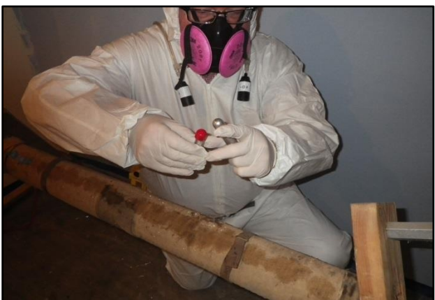
13. After putting the sample in the collection vial, each one was sealed air tight with a red rubber cap that is part of the book sampling system.
